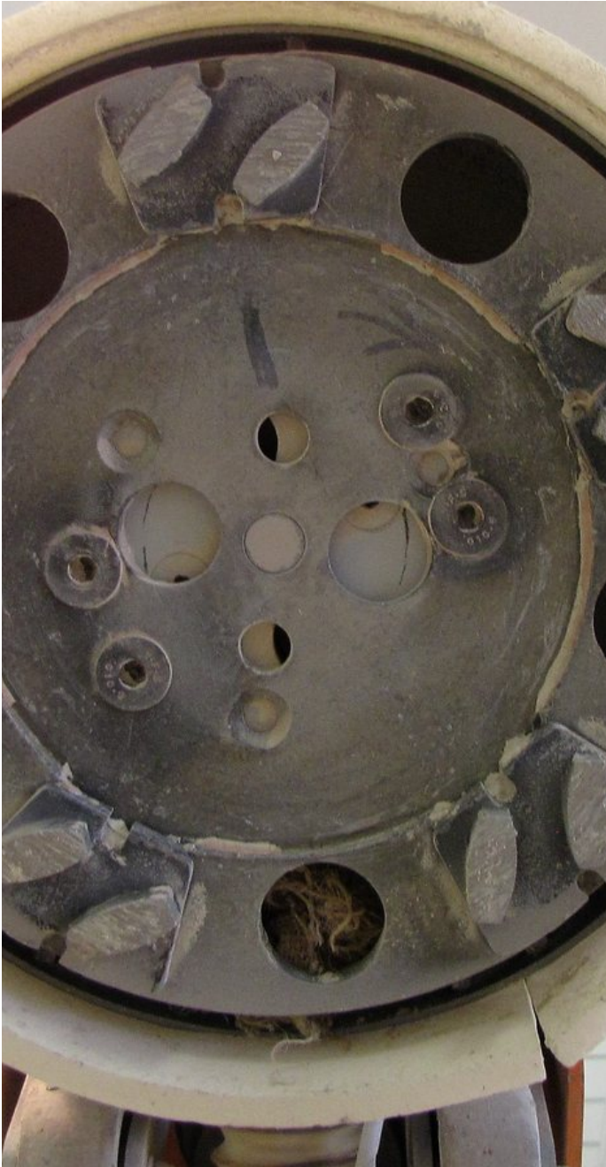
Single Header 3 Phase concrete grinding machine
